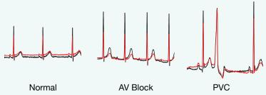
Evaluation on multiple subjects with different ECG morphologies. Simultaneous recordings from wet (black) and the Cognionics (red) sensor.
