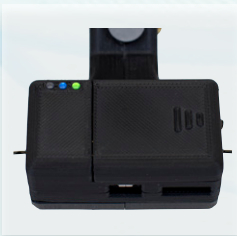
Step 2: Check wireless link quality indicator on headset to guarantee adequate signal and timing.
